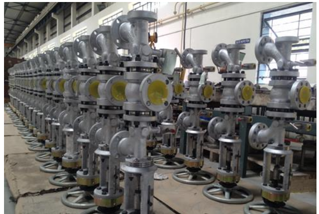
Changeover valves in the workshop
